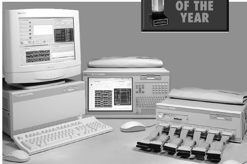
Figure 1. (left to right) The HP 16700A, 16702A and 16600A logic analysis systems.
